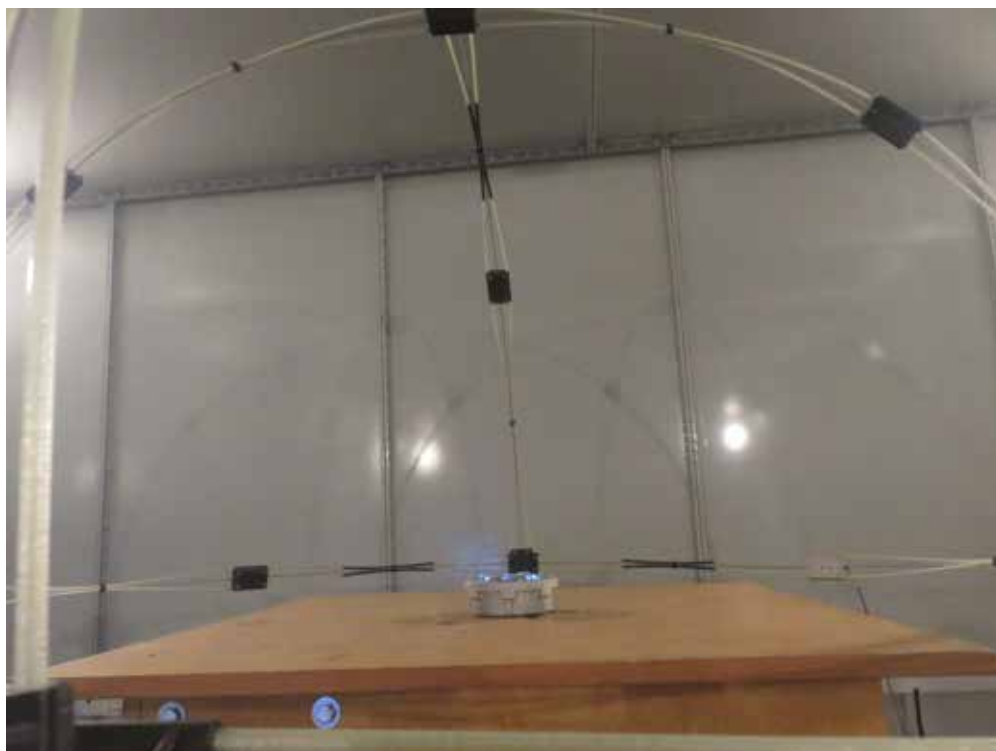
Photograph 4: Set-up for Radiated electromagnetic disturbances
