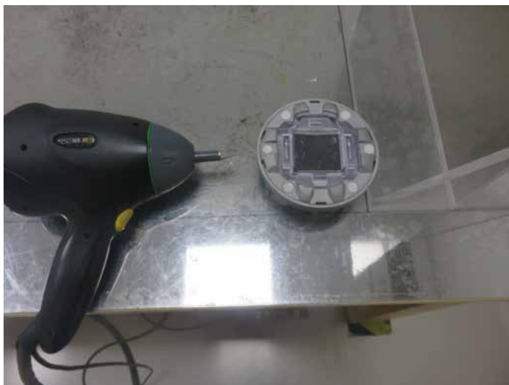
Photograph 2: Set-up for Electrostatic Discharge
