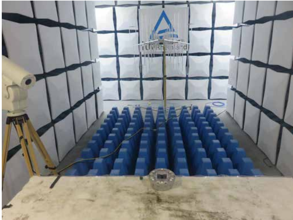
Photograph 4: Set-up for Radiated electromagnetic disturbances
